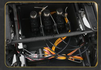
3-shift servos come pre-installed to control the 2-speed transmission (2WD or 4WD) and front/rear selectable differential lockers.
