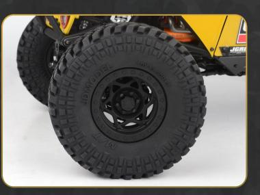
2-piece Beadlock Wheels are made from durable material, ensuring they can withstand the harshest terrains, and are scale recreations of the 1:1 set.
