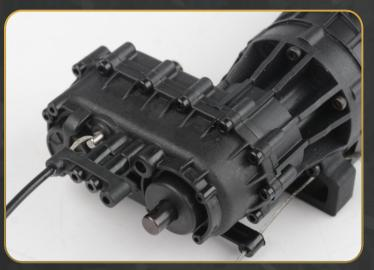
With a 2-speed transmission, switching from crawling over rocky terrain to racing across flatlands is quick at the push of a button.
