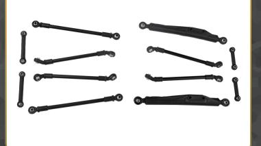
The front suspension has a traditional 4-link, while the rear sports a trailing arm setup with sway bars at the front and rear.
