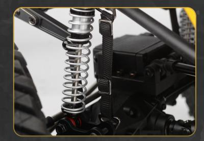
Like the full-size racer, there are front and rear sway bars and adjustable limiting straps on all four corners!
