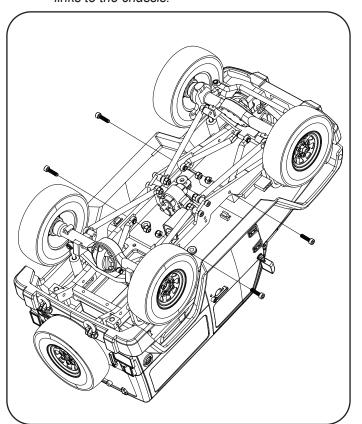
**Step 2.** Reverse the direction of the screw and reattach the upper links and sliders simultaneously. The nuts are not needed.
