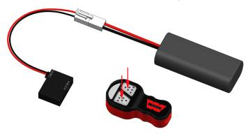
7. Plug in winch plug wire into control box and check operation of the winch.
