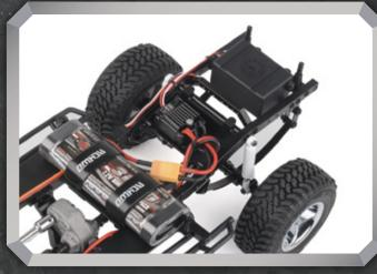
The Trail Finder 2 "LWB" Chassis has a multi-purpose, molded fuel cell that serves as an electronics storage box and provides additional RC realism by storing away any protruding wires.
