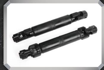
The driveshafts found on the Trail Finder 2 "LWB" Chassis feature heavy-duty uni-joint metal shafts for great driveline angles and durability on the trail.
