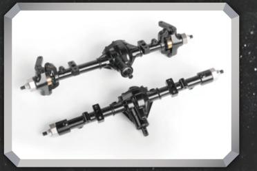
The most scale-accurate axles on the market, the K44 Ultimate Scale Cast Axles feature high steer knuckles, XVDs, lower mounting points, and a compact offset front pumpkin.
