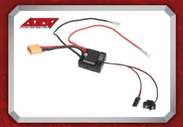
Included is the popular RC4WD Outcry III Waterproof ESC Brushed Speed Controller, with built-in drag brake, for reliable constant power on demand at any time!
