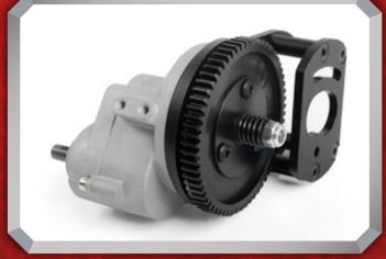
The R3 Single Speed Transmission comes with a tough cast metal case and wider gears for durability and a Delrin Spur with Slipper Clutch for performance. It also features a sturdy billet aluminum motor mount for added toughness.
