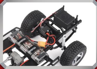
The Trail Finder 2 "LWB" Chassis has a multi-purpose, molded fuel cell that serves as an electronics storage box and provides additional RC realism by storing away any protruding wires.
