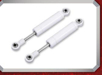
The Trail Finder 2 "LWB" Chassis includes Super Scale 70mm White Shocks with Internal Springs. These ultimate scale shock absorbers offer realistic looks and ultimate performance. They are machined from billet aluminum with internal springs and are customizable.
