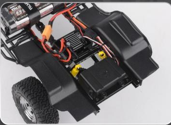
The Trail Finder 2 "LWB" Chassis has a multi-purpose, molded fuel cell that serves as an electronics storage box and provides additional RC realism by storing away protruding wires.
