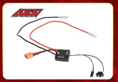
The 4Runner RTR features the popular RC4WD Outcry III Waterproof ESC Brushed Speed Controller with built-in drag brake for reliable, constant power on demand. Anytime.
