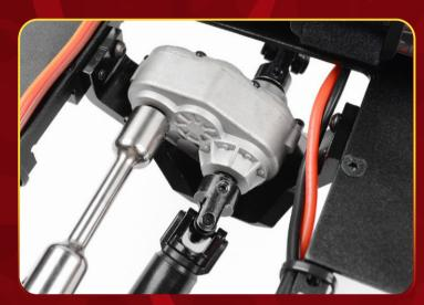
The 4Runner RTR includes the Hammer Transfer Case. Packed with detail, the Hammer features a cast metal exterior and heavy duty .8 Mod widened gears for durability.
