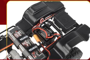
The 4Runner RTR Chassis features a molded fuel cell that doubles as an electronics storage box plus an aluminum frame mounted under cab electronics tray for multiple electronics mounting options.
