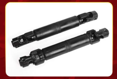
The Punisher Shafts for the TF2 feature bulletproof steel universals and a high quality plastic shaft for great driveline angles and durability on the trail.
