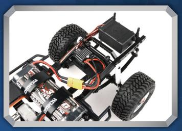
The Trail Finder 2 Long Wheel Base Chassis has a multi-purpose, molded fuel cell that serves as an electronics storage box and provides additional RC realism by storing away any protruding wires.
