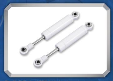
The Trail Finder 2 RTR includes Super Scale 70mm White Shocks with Internal Springs. These ultimate scale shock absorbers offer realistic looks and the ultimate in performance. They are machined from billet aluminum with internal springs and are rebuildable.
