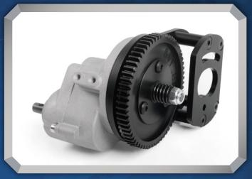
The R3 Single Speed Transmission comes with a tough cast metal case and wider gears to allow for more abuse along with a Delrin Spur with Slipper Clutch. It also features a sturdy billet aluminum motor mount for durability.
