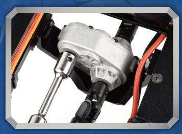
The Trail Finder 2 RTR includes the Hammer Transfer Case. Packed with scale detail, the case features a cast metal exterior and heavy duty .8 Mod Widened Gears for durability.
