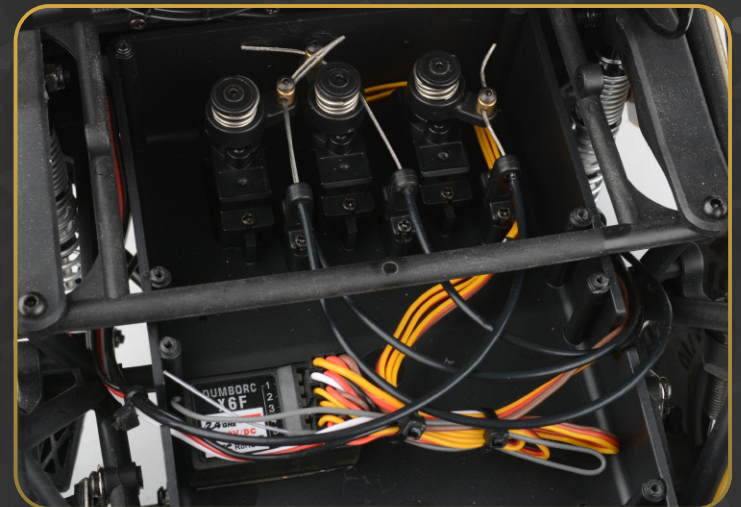
3-shift servos come pre-installed to control the 2 speed tranny, 2WD or 4WD and front/rear selectable differential lockers.
