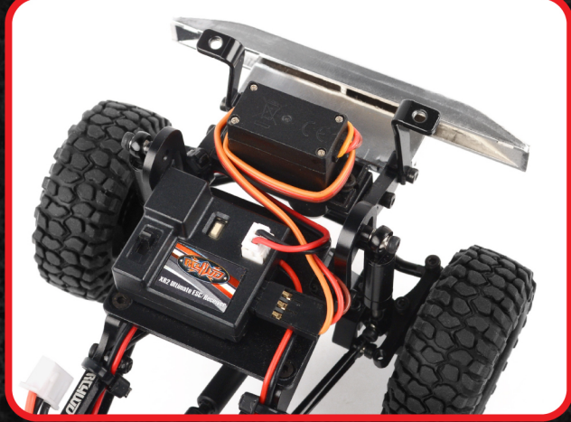
The G2 Chassis features a simple front mounted electronics plate for easy mounting of the XR2 Micro ESC/Receiver combo.
