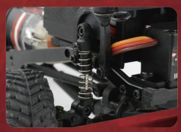
This RC suspension has a 4 link front and rear setup, allowing for some impressive shock absorption. These coil over shocks deliver the balanced driving needed for terrain stability!
