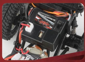
The 1/24 TF2 chassis features a simple front mounted electronics plate for easy mounting of the XR2 Micro ESC/Receiver combo.
