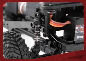
This RC suspension has a 4 link front and rear setup, allowing for some impressive shock absorption. These coil over shocks deliver the balanced driving needed for terrain stability!
