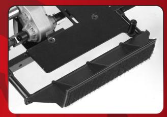
Velcro is included to secure the sides of the body to the chassis, providing extra rigidity to the body.
