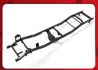
With solid strength in mind, the ladder frame design of the TF2 Long Wheel Base Chassis is made with CNC machined, billet aluminum and comes with scale shock hoops, a chassis servo mount and transmission and transfer case mounts.
