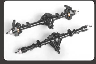
The most scale-accurate axles in the market, the **RC4WD Yota II Ultimate Scale Cast Axles feature** innovative round knuckles, lower mounting points, XVDs for the front axles and compact offset pumpkins.
