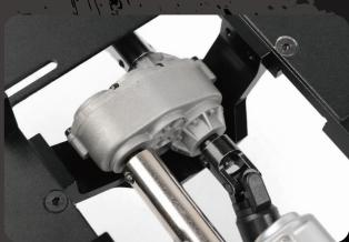
The Trail Finder 2 LWB Kit includes the Hammer Transfer Case. Packed with detail, the case features a cast metal exterior and the same 0.8 Mod widened gears for durability.
