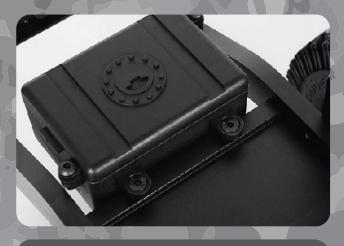
The G2 Chassis features a molded fuel cell that doubles as an electronics storage box. There is also an aluminum, frame-mounted under cab electronics tray for multiple electronics mounting options!
