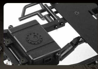
The TF2 LWB Kit Chassis features a molded fuel cell that doubles as an electronics storage box and an aluminum, frame mounted under cab electronics tray for multiple electronics tray for multiple mounting options for your electronics.
