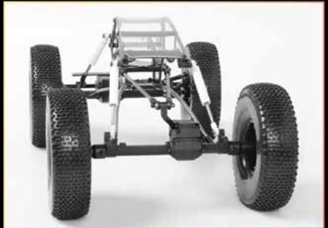
The new Bullseye 2 Gear Set is installed on Bullseye 2 Competition Crawler Axles. They have the most durable gears RC4WD has ever offered so that the MOA will stay on the rocks, day after day.
