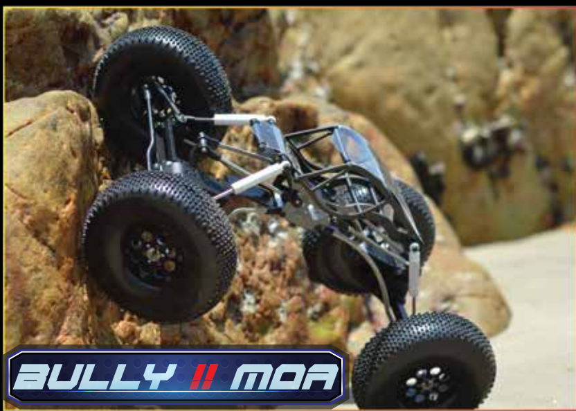
These solid titanium links are made from RC4WD and offer great drive-line angles and performance on the rocks.
