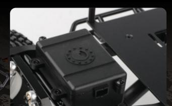
The TF2 Chassis features a molded fuel cell that doubles as an electronics storage box plus an aluminum, frame-mounted under cab electronics tray for multiple electronics mounting options.
