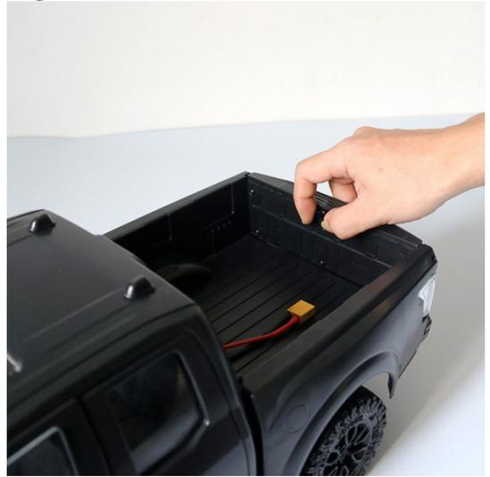
Squeeze the mechanism on the inside of the tailgate with your fingers.
