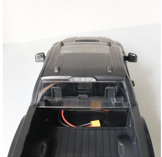
Step 2. Pull the rear cab back out and away from the truck bed.
