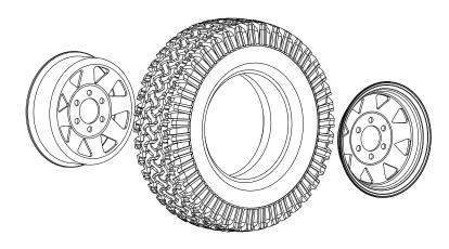
4: Use the included longer hardware to help aid in tire and wheel installation. Be sure to slowly tighten the nuts on the longer hardware until you are able to begin installing the include shorter hardware. 5: Install the correct shorter length hardware into the remaining holes.
