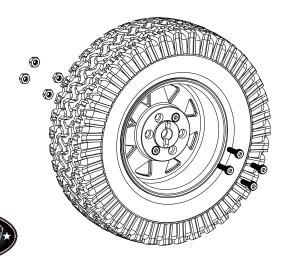
6: Begin to tighten the hardware in a star shape pattern to fully seat the tire to the wheel properly.
