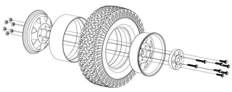
2: Insert internal beadlock ring Into tire.
